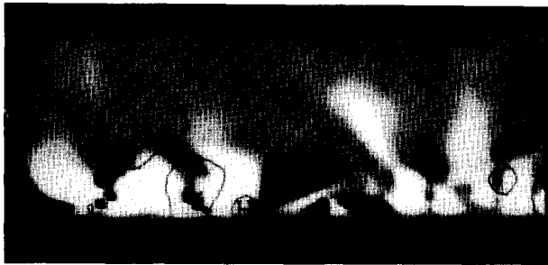
Figure 16 Production for \overline{u'^2} in the y - z plane: gray to black, -2\overline{u'v'}(\partial\overline{u^+}/\partial y^+) = 0 to -0.4 ; gray to white, -2\overline{u'v'}(\partial\overline{u^+}/\partial y^+) = 0 to +0.4
