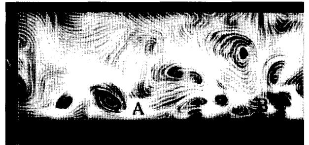
Figure 7(a) Instantaneous streamlines and second invariant of the deformation tensor II in the y - z plane: gray to black, u'_{i,j} u'_{j,i} = 0 to -0.02 ; gray to white, u'_{i,j} u'_{j,i} = 0 to +0.02
