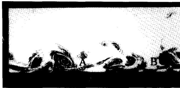
Figure 5(b) Instantaneous streamlines and enstrophy in the y - z plane: white to black, \omega_i^+ \omega_i^+ = 0 to 0.05
